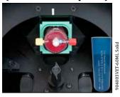
Push Open/Stop button on control panel. The "unlocked" indicator will illuminate. Turn latch counterclockwise to open lid. Place *Restigen* Device into centrifuge. Be sure the centrifuge is balanced with counterbalance (Part # 904003VET-60ML Solid (shown) or 904001VET-60ML) or second full *Restigen* Device.
