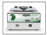
Close lid by rotating the lid latch clockwise. "Latched" indicator will illuminate. Set speed to 3200 RPM and time to 15 minutes. Press Start button. Once spin is complete, press Open/Stop button. Twist latch counterclockwise to open lid.
